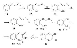
i = n-BuLi, THF, -10°C; ii = Se; iii = aq NH<sub>4</sub>Cl; iv = MeOH, NaOH (cat.), O<sub>2</sub>; v = MeOH, H<sub>2</sub>O, HCl, 60°C; vi = PrNCO, 70°C; vii = (PhCOO)<sub>2</sub>, benzene, 80°C
