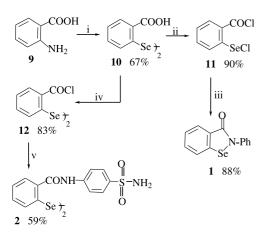
i = 1. NaNO<sub>2</sub>, HCl,  $-5^{\circ}$ C; 2. Na<sub>2</sub>Se<sub>2</sub>; ii = SOCl<sub>2</sub> (excess), DMF (cat.) reflux; iii = PhNH<sub>2</sub>, MeCN; iv = SOCl<sub>2</sub>, benzene, reflux; v = 4-NH<sub>2</sub>C<sub>6</sub>H<sub>4</sub>SO<sub>2</sub>NH<sub>2</sub>, toluene, pyridine, reflux.
